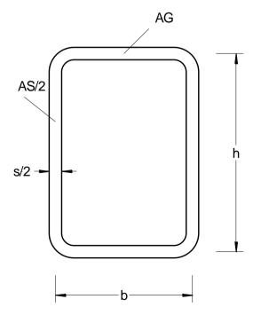
For RHS section, classified as Plastic-Plastic or Elastic-Plastic, the plastic interaction formula according to Ref.[13], can be selected.
